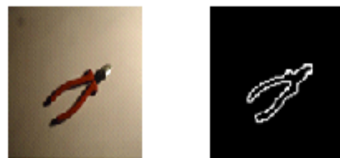
Fig. 1. Preprocessing of the input RGB image. a) RGB image of a plier, b) preprocessed binary image with edges shown in white.
