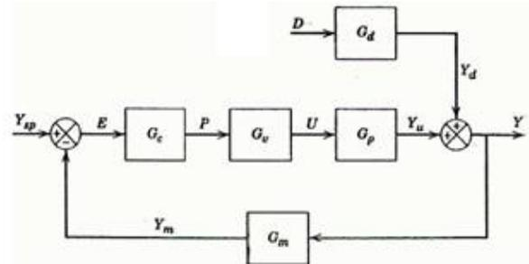
Figure 2: Standard feedback control system representation.
