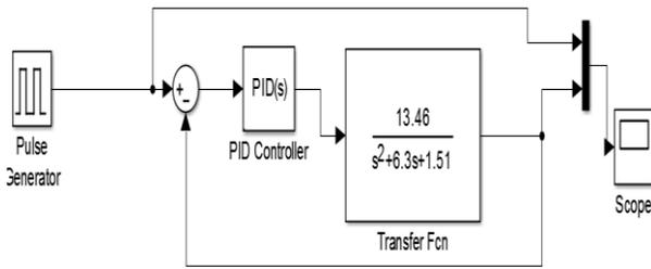
Figure 3: Simulation model in programming environment.
